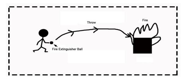
(Active Use) Throwing Fire Extinguishing Ball into the fire - When a fire erupts, take the nearest available Fire Extinguishing Ball and simply throw it into the fire. The ball will naturally fall into the base of the flame, where it is most needed, and activate within 3 seconds. No need to pull pins, or to get close to the fire. No special training or skills required.
