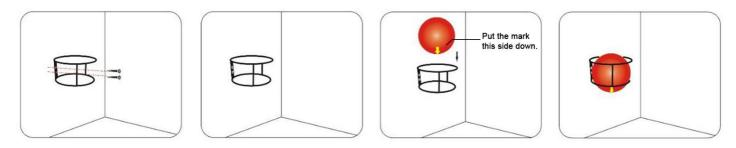
(Passive Use) Self Activating Mount – One of the great benefits of Fire Extinguishing Ball is the fact that it can self activate in the presence of fire when no-one is present. If positioned in the appropriate high-risk area where most fires are likely to start, it will self activate upon reaching the appropriate temperature and extinguish the fire.
